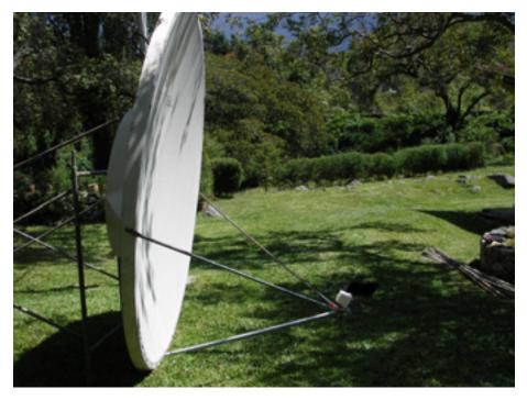
Figure 11.29: 2.4 m offset fed reflector with a 12 dBi antenna at its focus, looking 14° down. The actual elevation is 8° up.
