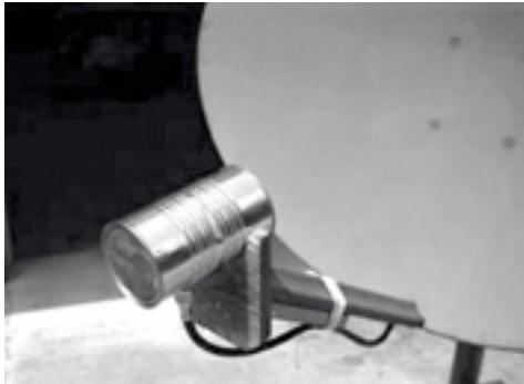
Figure 4.10: Feed horn made from a food can.
