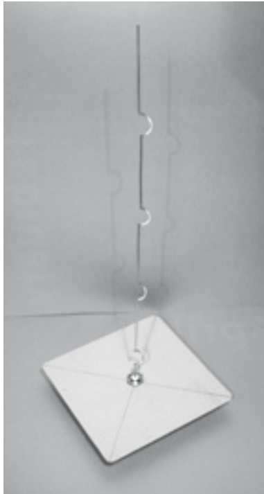
Figure 4.29: The finished antenna should be 42.5 cm from the plate to the end of the wire.
