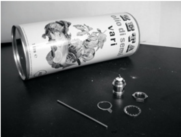
Figure 4.33: Parts needed for the can antenna.
