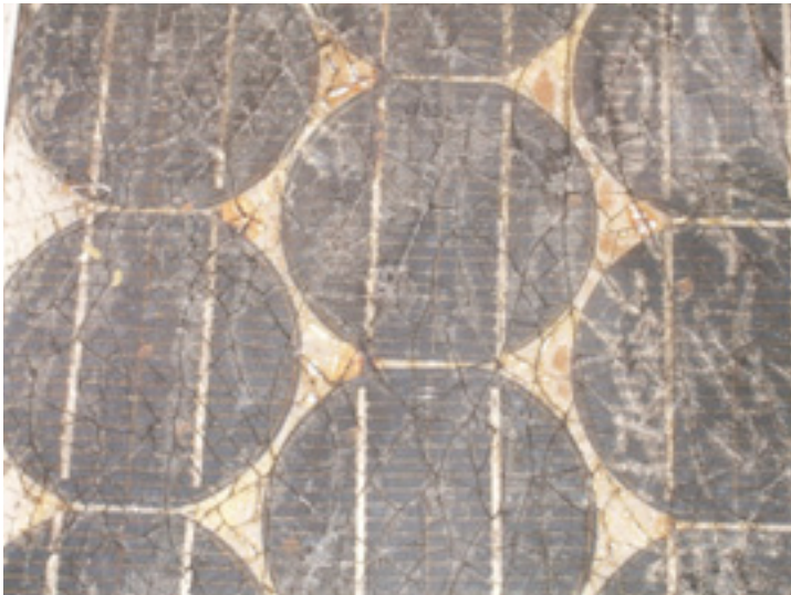
Figure 7.6: The effect of water and corrosion in a solar panel
