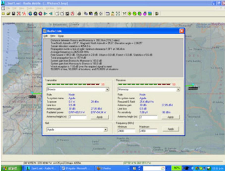
Figure 11.28: Propagation details of the 280 km link.
