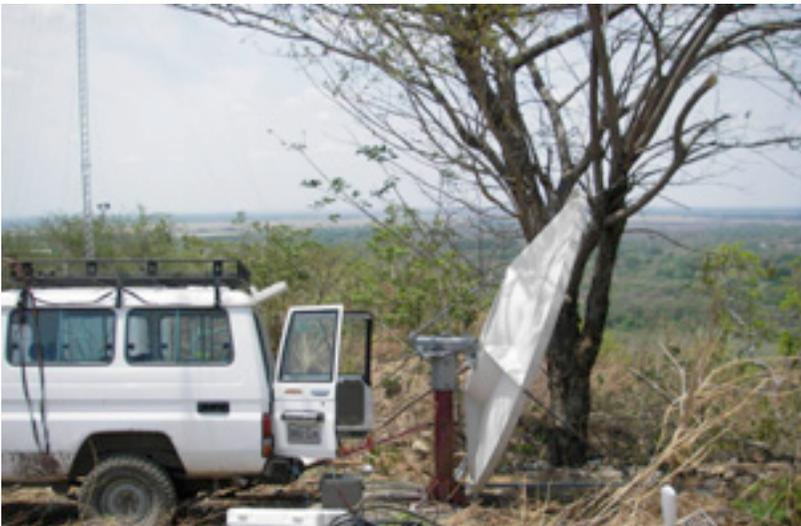
*Figure 11.34: El Baúl antenna installation. Actual elevation was  $1^\circ$  upward, since the antenna has an offset of  $22.5^\circ$ .*
